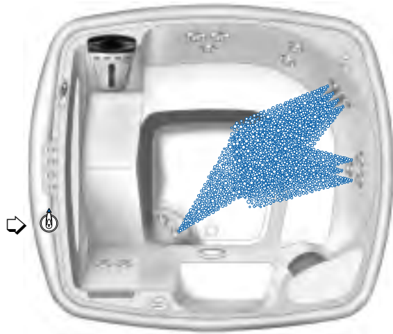
Left Jet Pump–Jet System 1 Left SmartJet® Lever in the 3 o'clock position
