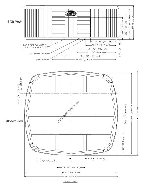
NOTE: Watkins Mfg. Corp. recommends the LANDMARK be installed on 3" (7.6 cm) to 4" (10 cm) reinforced concrete pad. WARNING: The LANDMARK can not be shimmed in any manner.
