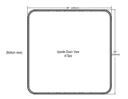
**NOTE:** Watkins Manufacturing Corporation recommends that the Pulse be installed on a minimum 4" thick reinforced concrete pad or structurally sound deck able to support the "dead weight" found in the spa specification chart.
