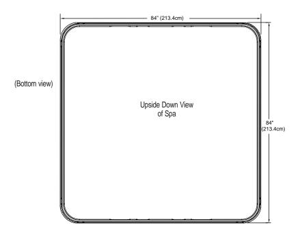
**NOTE:** Watkins Manufacturing Corporation recommends that the Flair be installed on a minimum 4" thick reinforced concrete pad or structurally sound deck able to support the "dead weight" found in the spa specification chart.
