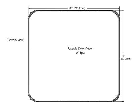
**NOTE:** Watkins Manufacturing Corporation recommends that the Bolt be installed on a minimum 4" thick reinforced concrete pad or structurally sound deck able to support the "dead weight" found in the spa specification chart.
