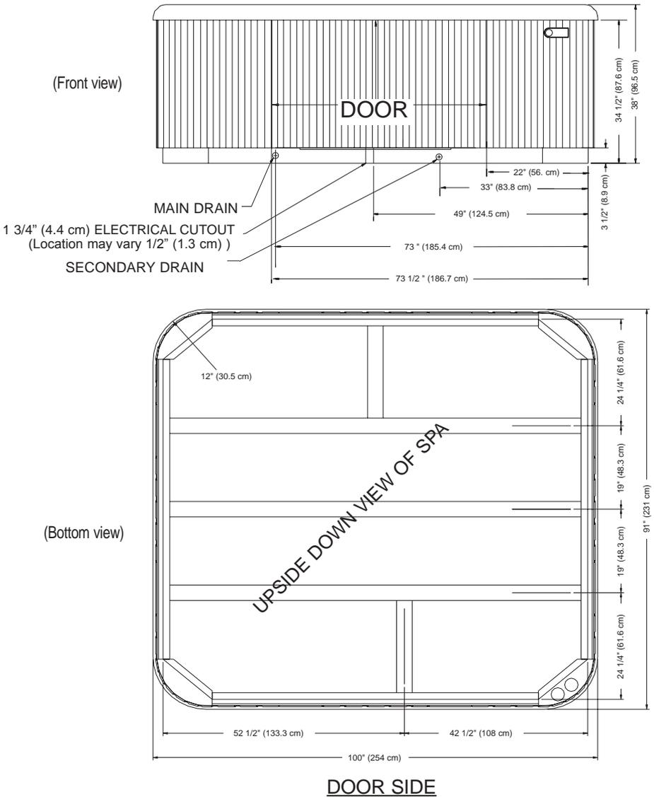
**NOTE:** Watkins Manufacturing Corporation requires that the Vista be installed on a minimum 4" thick reinforced concrete pad or a deck that is able to withstand more than 115 lbs. per square foot.
