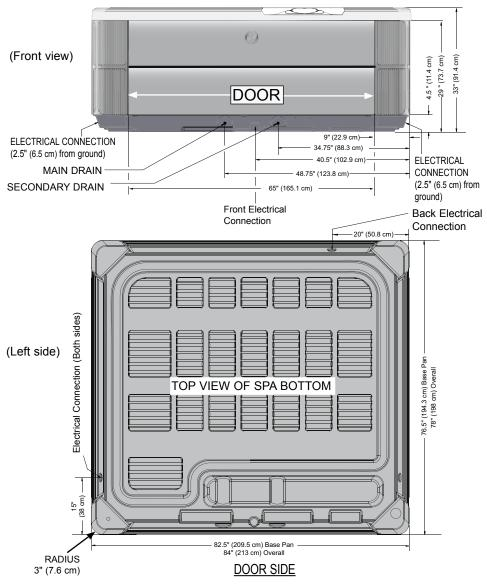
**NOTE: WATKINS WELLNESS** recommends that the **PRODIGY** be installed on a minimum 4" (10 cm) thick reinforced concrete pad or a deck that is able to withstand more than 130 lbs/ft<sup>2</sup> (620 kg/m<sup>2</sup>).
