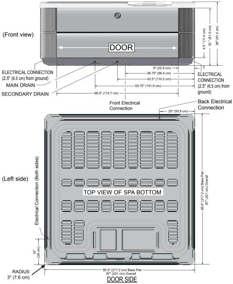
**NOTE: WATKINS WELLNESS** recommends that the **VANGUARD & ARIA** be installed on a minimum 4" (10 cm) thick reinforced concrete pad or a deck that is able to withstand more than 130 lbs/ft<sup>2</sup> (630 kg/m<sup>2</sup>) & 125 lbs/ft<sup>2</sup> (595 kg/m<sup>2</sup>).
