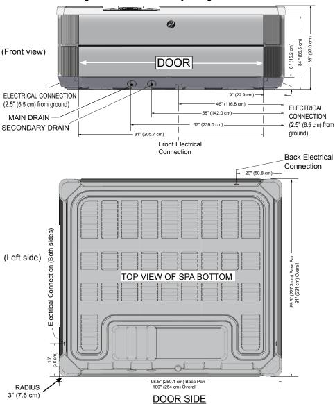
**NOTE: WATKINS WELLNESS** requires that the **GRANDEE** be installed on a minimum 4" (10 cm) thick reinforced concrete pad or a deck that is able to withstand more than 125 lbs/ft<sup>2</sup> (605 kg/m<sup>2</sup>).
